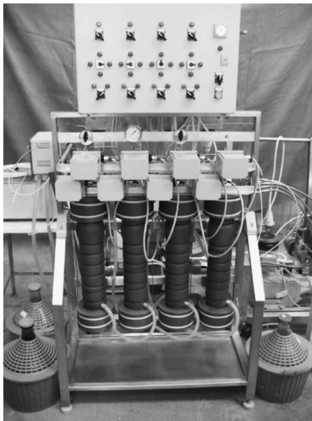
Fig. 3. The photograph of the SMB equipment. The four jacketed stainless steel columns are in thermal isolation. Four pieces two position cocks and four pieces four position cocks are actuated by a PLC. Two pieces of two position manual cocks given for degassing.
